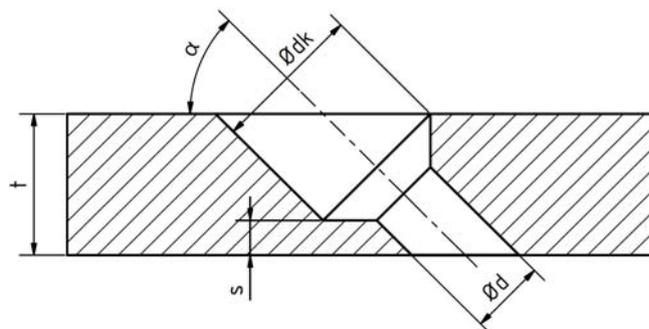
$\alpha \geq 45^\circ$        $s \geq 3 \text{ mm}$
