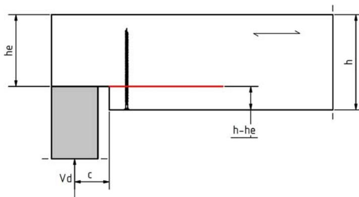
Tension reinforcement of openings may be designed according to
