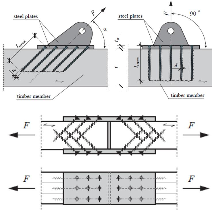
Sufficient contact of the screw head must be ensured. This is fulfilled for countersunk heads with countersunk washer as well as heads with a flat bottom side (e.g. pan head, washer head, SuperSenkFix,...) for 90° drillings. Alternatively, countersunk head screws may be used in 90° countersunk drillings where
