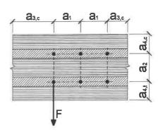
A.2.2 Definition of spacing, end and edge distances in the edge surface of the cross laminated timber. For screws in the edge surface, a1 and a3 are parallel to the CLT plane face, a2 and a4 perpendicular to CLT plane face.
